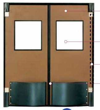
Door Panel - Lightweight, weighing only 2.5 pounds per square foot, is easy to open, operates smoothly and allows for safe passage of personnel and damage free equipment. The overall panel thickness is 1-7/8", the skin thickness is 1/8" thick and the door can be sized up to a 8' x 10'. Rotationally molded polyethylene outer skin retains its properties to -40°F.
