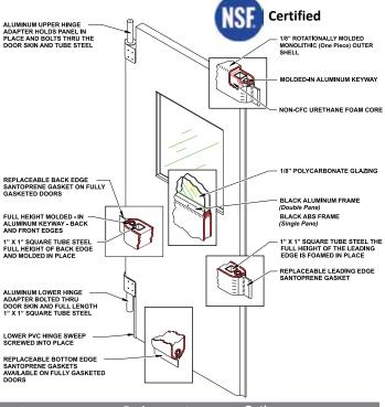
**Insulated Core** – The foamed-in-place Non-CFC urethane core (permanently bonded to the outer surface) does not break down when impacted, provides noise control and provides excellent insulation with an R factor of 10.83.
