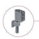
**Bottom Hinge** – For additional strength and durability the hinge is designed with pillow block constructed of zinc plated ductile iron (stainless steel is optional) with a UHMW sleeve and solid cast aluminum lower hinge adapter. Plus the lower hinge adapter has a provision for mounting an optional spring assist.
